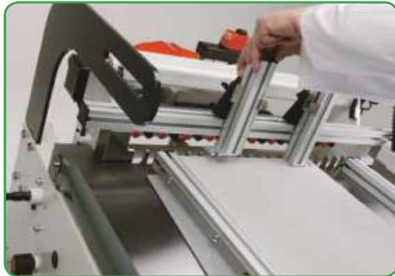
Device to automatically change the vertical horizontal depth (-10mm) to avoid chipping of the panel
