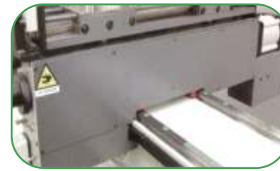
Linear guideways for Vertical Drill Head positioning
