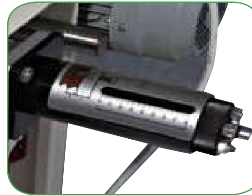
Revolver with 6 positions for boring depth setting
