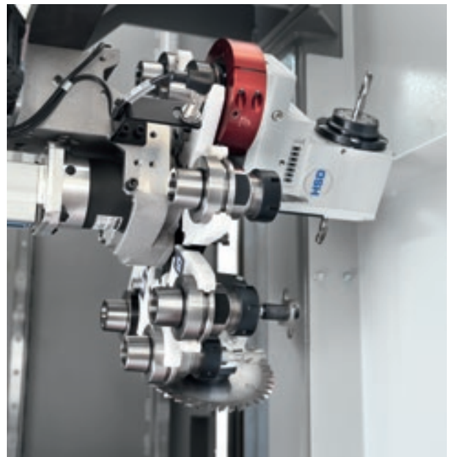
8-position tool magazine that manages different types of aggregates, thus increasing the machine's versatility.
