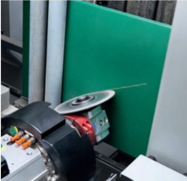
Cutting machine with integrated C-axis (optional).
