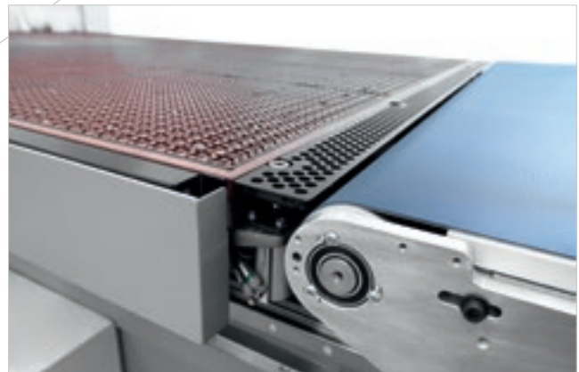
Dust intake manifold between machine and unloading belt.
