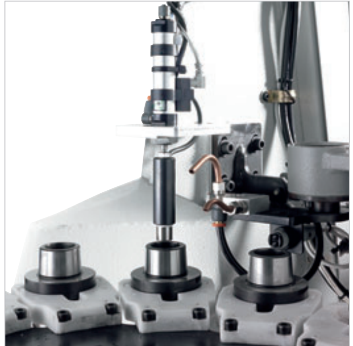
Chip reading system integrated in the tool holder, for automatic tool recognition.
