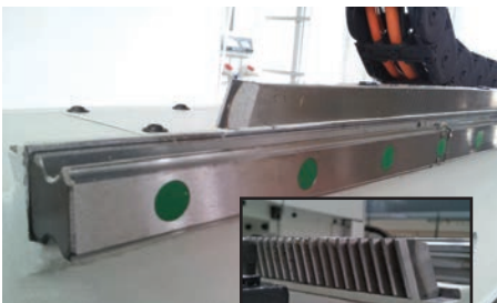
Y Axis linear guide and Helical rack
