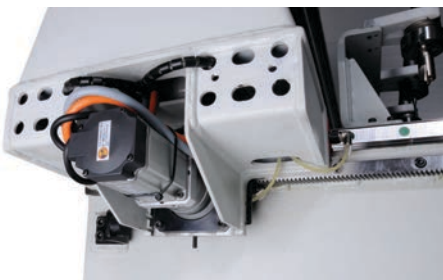
X Axis helical rack & pinion with precision linear guides and digital servo motors guarantee high precision and high quality cut
