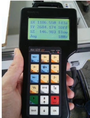
Easy to use DSP numerical control with handheld device
