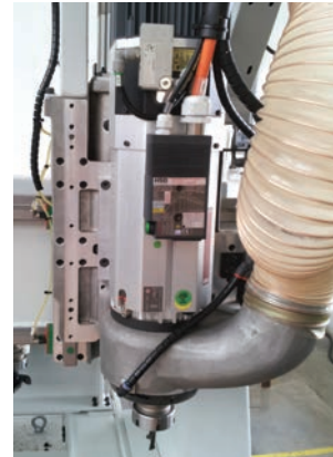
Powerful 15HP HSD Electro-spindle, ISO or HSK
