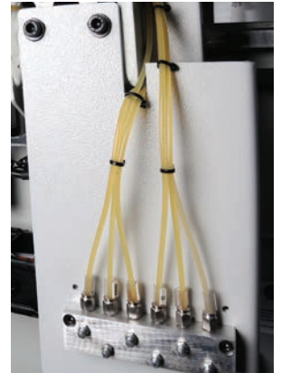
Central Lubrication makes maintenance simple
