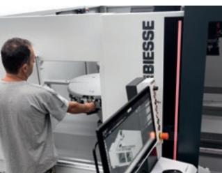
With one 16-position **revolving warehouse** which is easily accessible from the front as standard, a second optional 16-position warehouse can also be added, for a total of 32 tool spaces.
