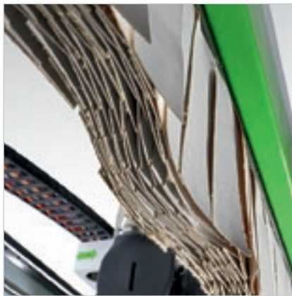
Side curtain guards to protect the working unit; they can be moved to enable the machine to work at maximum speed in total safety.
