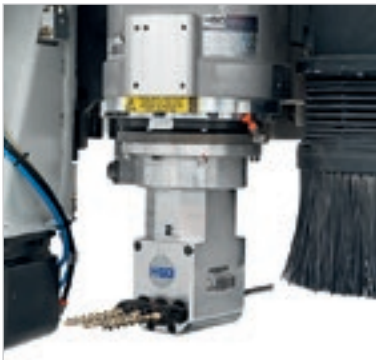
The NC controlled multi-function unit can be infinitely positioned on a 360 (degree) rotation. It can also be used to house aggregates for specific machining operations such as pocketing for locks, hinges, deep horizontal holes and edge-trimming.
