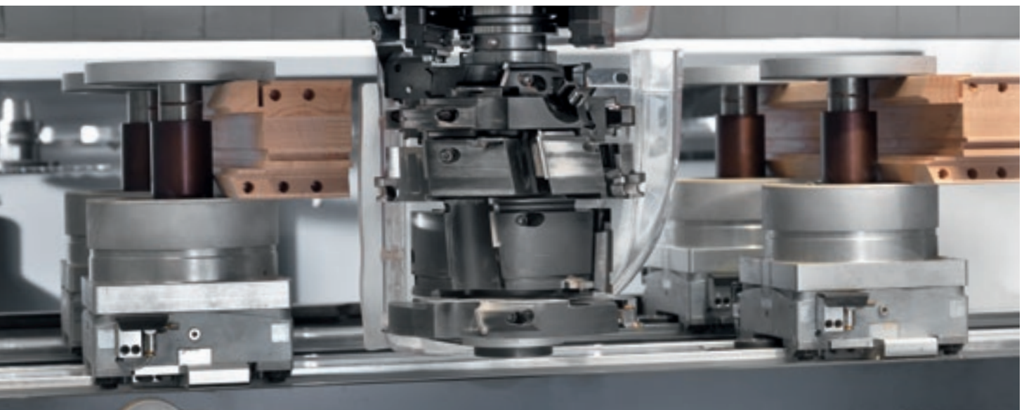
Uniclamp and Hyperclamp pneumatic locking systems with quick release, for firm and precise locking.
