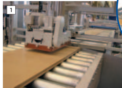
1 Decklagen beschicken Top-layer infeed
