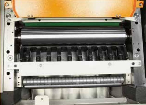
Planer unit with infeed anti kick-back fingers and segmented chipbreakers, serrated steel infeed roller with spiral teeth and rubber coated outfeed roller. Reduced noise level.
