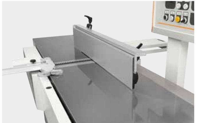
The additional overturning fence, available on request, is recommended to machine thin workpieces
