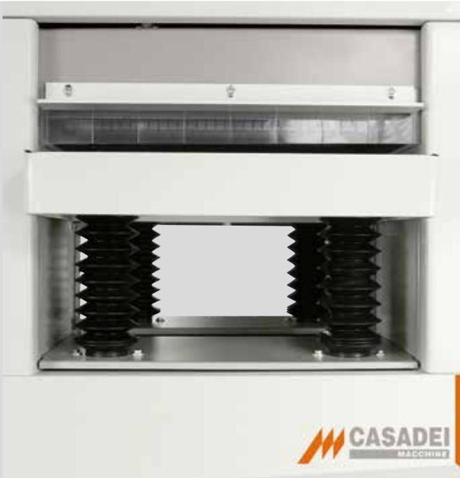
Powered 2 speeds thickening table raise & fall, with micrometric adjustment of the working height and 4 steel screws protected by dust. Noise reduction lips positioned at front and rear of machine table.
