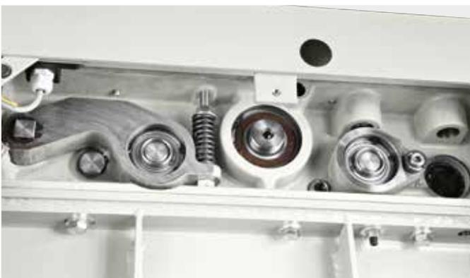
Feed rollers mounted on independent floating ball-bearing bushes.
