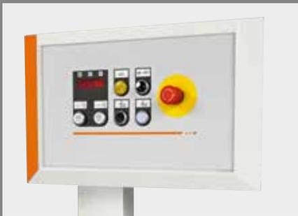
Ergonomics and easy of use. All electric controls are centralised and conveniently located in the main control cabinet.
