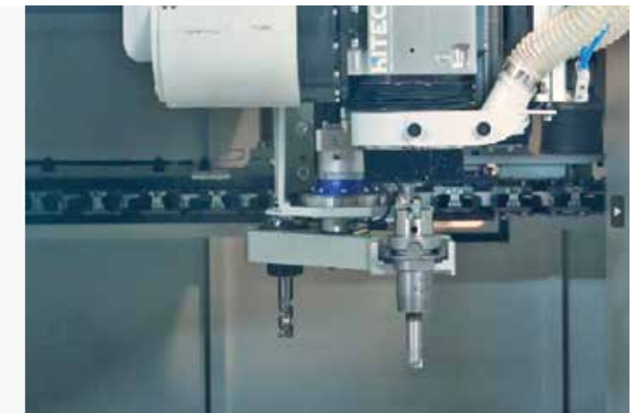
Tool-chain magazine with exchange handgrip
