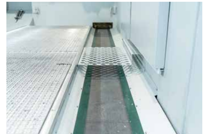
Chips management with integrated conveyor
