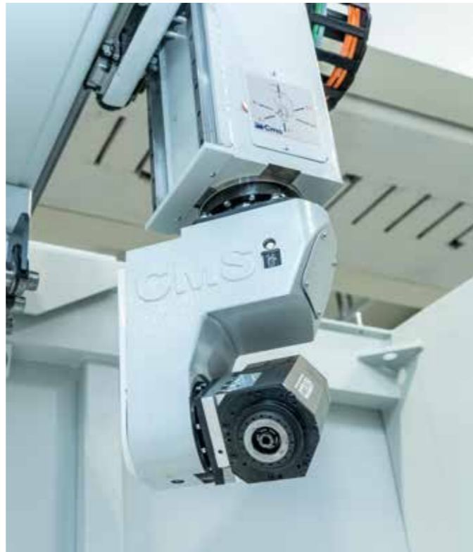
CX5 WORKING UNIT
