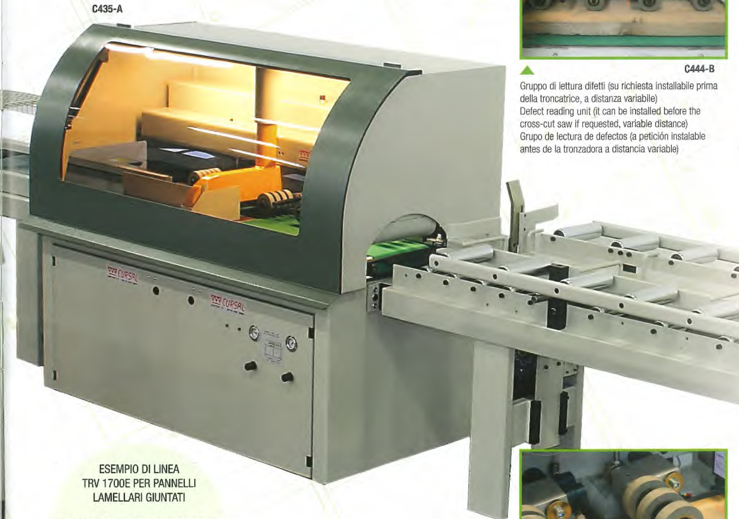
EXAMPLE OF A TRV 1700E LINE FOR LAMINATED, FINGER JOINED PANELS
