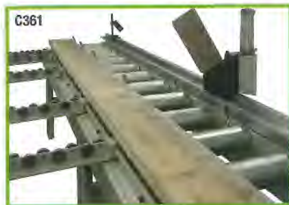
Ejection phases: 1- plank placed on the stop, 2- working levers 3- ejected plank
