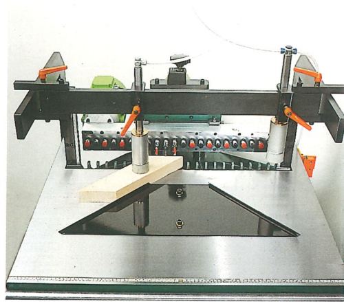
Horizontally drilling with a device for 45 degrees drilling
