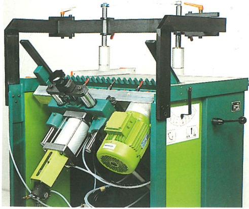
Drilling under any angle from 0 to 90 degrees
