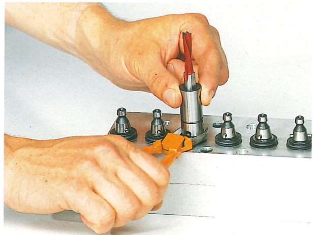
Drilling head with quick exchange chucks
