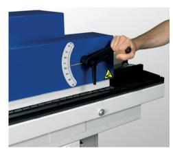
The height of the top pressure bar can be adjusted by a lever. This can be read easily thanks to a large scale.
