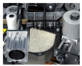
The 1.2 kg teflon coated glue pot is designed for EVA granulate glue. The glue is applied via an adjutable glue roller.
