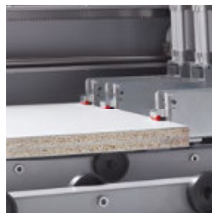
Saw carriage with main and scoring unit
