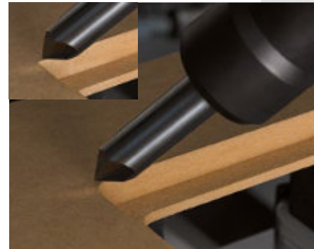
Sharpening of corners
