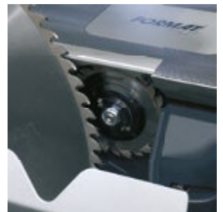
Tool free saw blade change system
