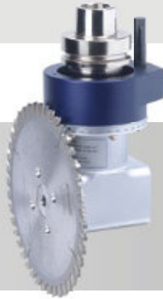
HSK F63 Single angle head, for use with a screw mounted saw blade with one WELDON connection, max. Ø 180 mm Order no. 300-24-002 max. Ø 240 mm Order no. 300-24-003 max. Ø 300 mm Order no. 300-24-007
