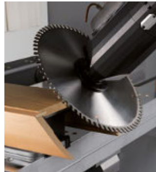
Door frame manufacturing
