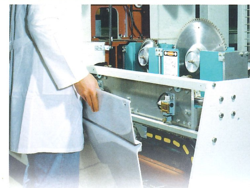
Side covers specially designed for noise reduction, allow easy access to all sections of the machine.
