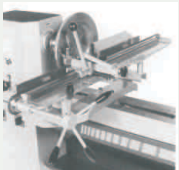
KA-90 with copying transversal support to copy plates, discs,...
