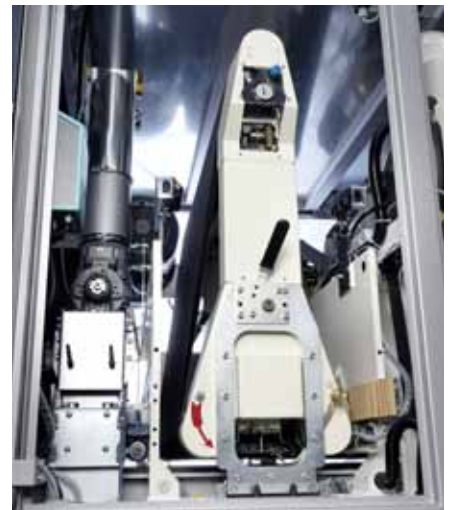
Longitudinal sanding unit (with or without pressure segment belt)
