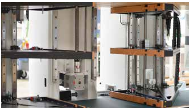
Lateral clamping plates: The clamping plates work as a unit. The pressing forces are generated electrically and can be adjusted individually. Pressure is applied vertically by a pressure plate and horizontally by the three clamping plates.
