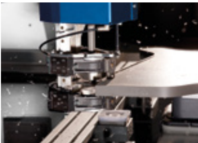
Perfect edge finish with traced combination flush trimming / scraping unit
