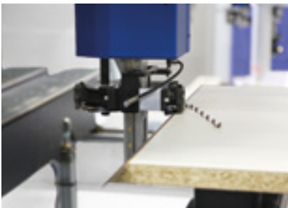
Scraping of mitered edges
