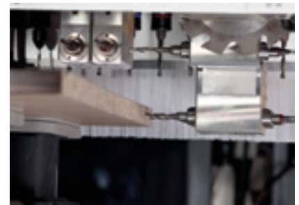
Horizontal boreholes for carcass connections
