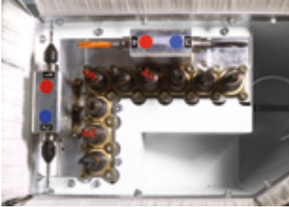
Drilling head V9/H4: HIGH-SPEED drilling head up to 7500 rpm with 9 vertical spindles and 4 horizontal spindles.
