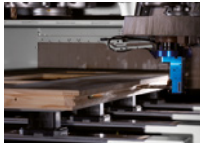
Lock case trimming on front doors
