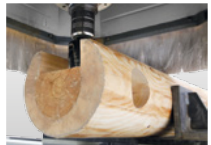
Block clamp: Adapted block clamping fixture for round timber elements.
