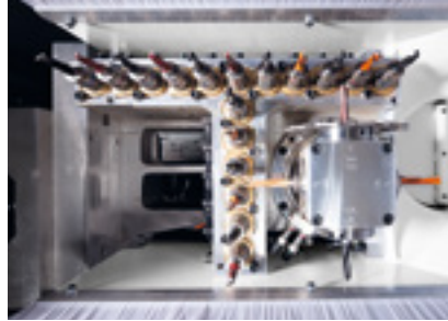
Drilling head V17/H4: HIGH-SPEED drilling head up to 7500 rpm with 17 vertical spindles, grooving saw and 4 horizontal spindles with 0/90° swivel facility. Fast drilling including grooving in the X/Y direction.
