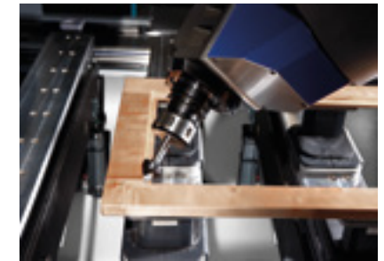
Square corner routing for a glass rebate
