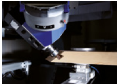
Routing of a dovetail joint for upright / transom constructions
