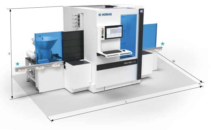
★ A corresponding safety distance must be maintained in the in and outfeed direction! (See documentation)
