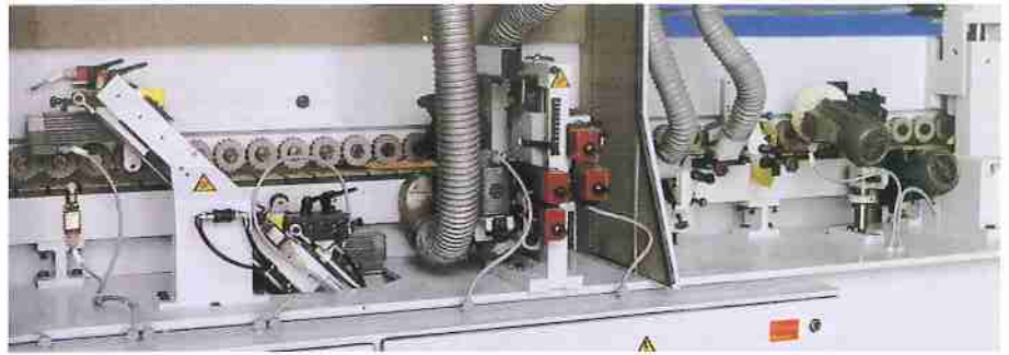
End trimming, Trimming, Scraping and Buffing
