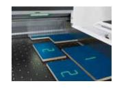
If destacking locations have been predefined, numbers appear on the finished workpieces. These correspond to a pallet number. The operator simply destacks the part to the corresponding pallet.
