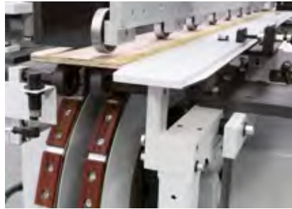
The rolling chain also ensures quiet running, even at high feed rates
