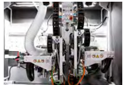
High-power trimming unit SF30 with automatic adjustments
