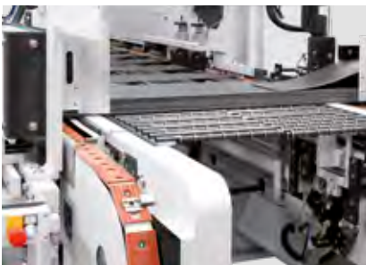
Intermediate magazine especially for LVT
