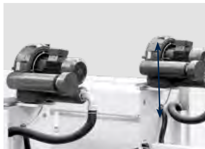
Chain track ventilation on both sides
