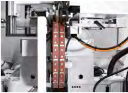
Tension-free infeed system with improved stability
