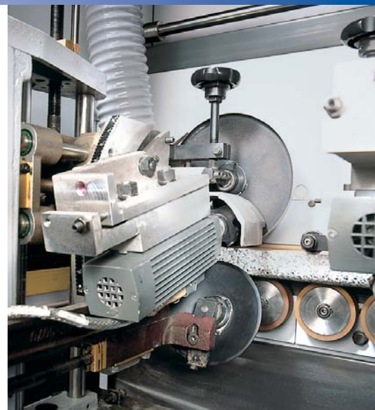
Trimming unit above for L profiles For chamfer trimming the overhanging laminate.
