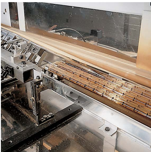
Heating lamps and pressure zone For thermal preparation / forming and pressing on the overhanging laminate.
