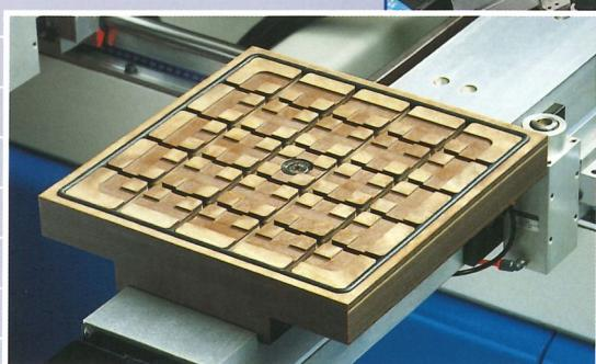
Spline vacuum cup to create part of spline matrix table.
