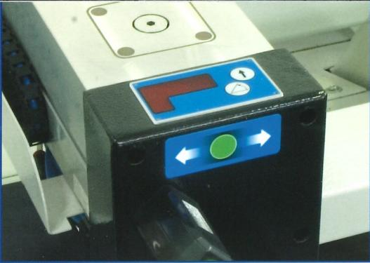
Digital display showing the data sent by the NC, related to the setting of the working table according to the job to be carried out.
