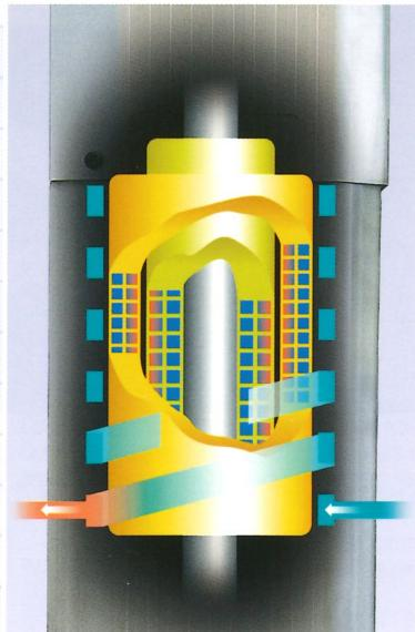
Liquid cooled electrospindles.
