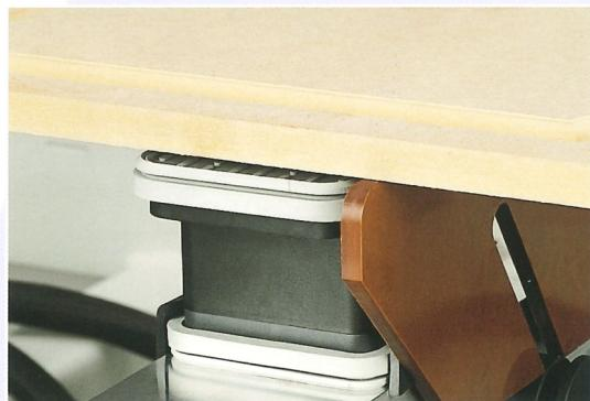
Panel lifting blades for easy positioning of heavy workpieces and NC controlled reference stops.
