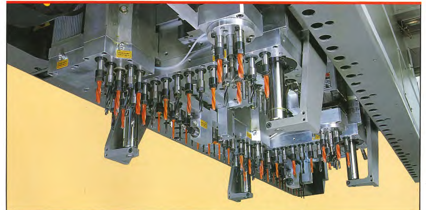
Vertical boring units with independent spindles
