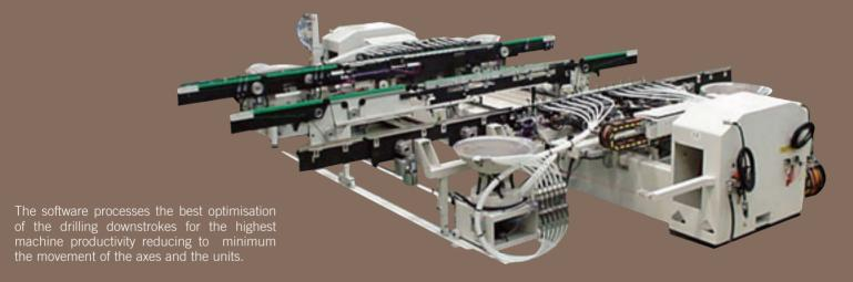
Unprecedented productivity and flexibility are guaranteed by a production line consisting of a drilling machine and inserter, controlled by a single software station.
