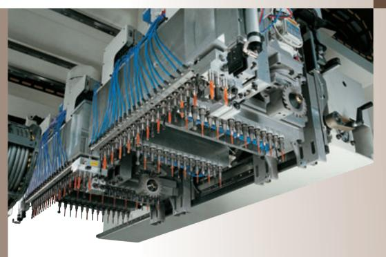
The vertical units (2 for FLEXA and 4 for AUTHOR 924) are mirroring each other. They have an independent stroke along the X, Y and Z axes and they are able to optimise the drilling, to reduce the panel machining times to a minimum.
