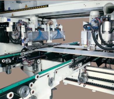
The panel conveyor continually adapts itself to the dimensions and the weight of the workpieces, thanks to an inverter that manages the speed up to 120 m/min.
