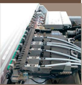
All the drilling and dowelling operations can be performed quickly, automatically and flexibly thanks to the modularity of the Flexa 912 and Author 924.
