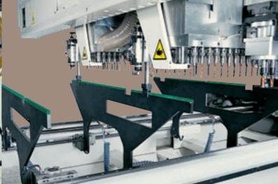
Displacement of the work tables managed by the numeric control. With the vertical unit a device picks up each single table and positions it at the desired quota, in a total time that can vary between 15" and 45".
