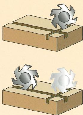
The unit is able to cut grooves along the X and Y axes, to square off even very thick panels (as blades of up to **200mm diameter** can be fitted) and to cut frames and workpieces in solid wood.
