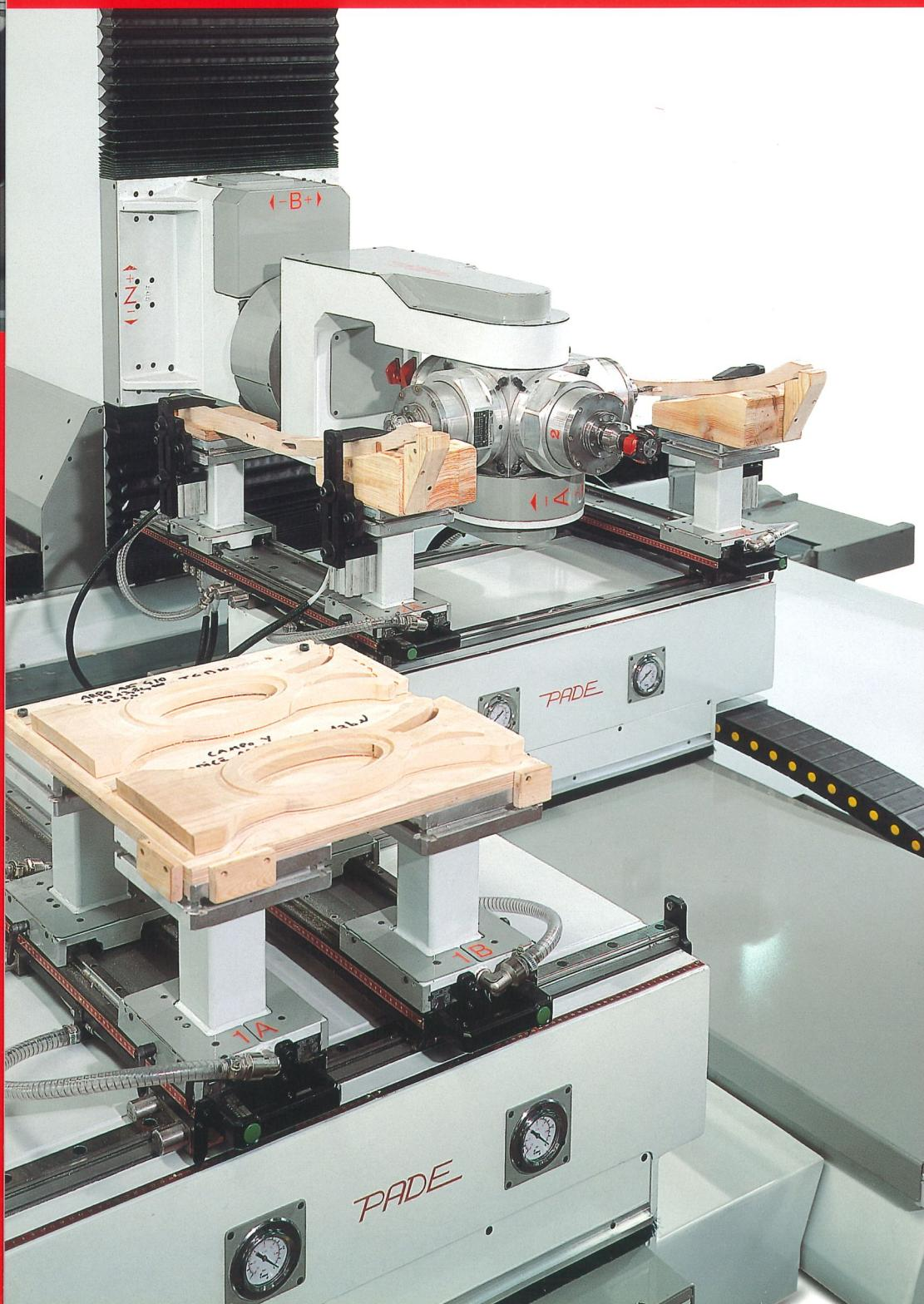
The two worktables offer the great advantage of either working on the full field surface (long pieces) or in alternate cycle. They are supplied with clamping cylinders and equipped for vacuum connection.
