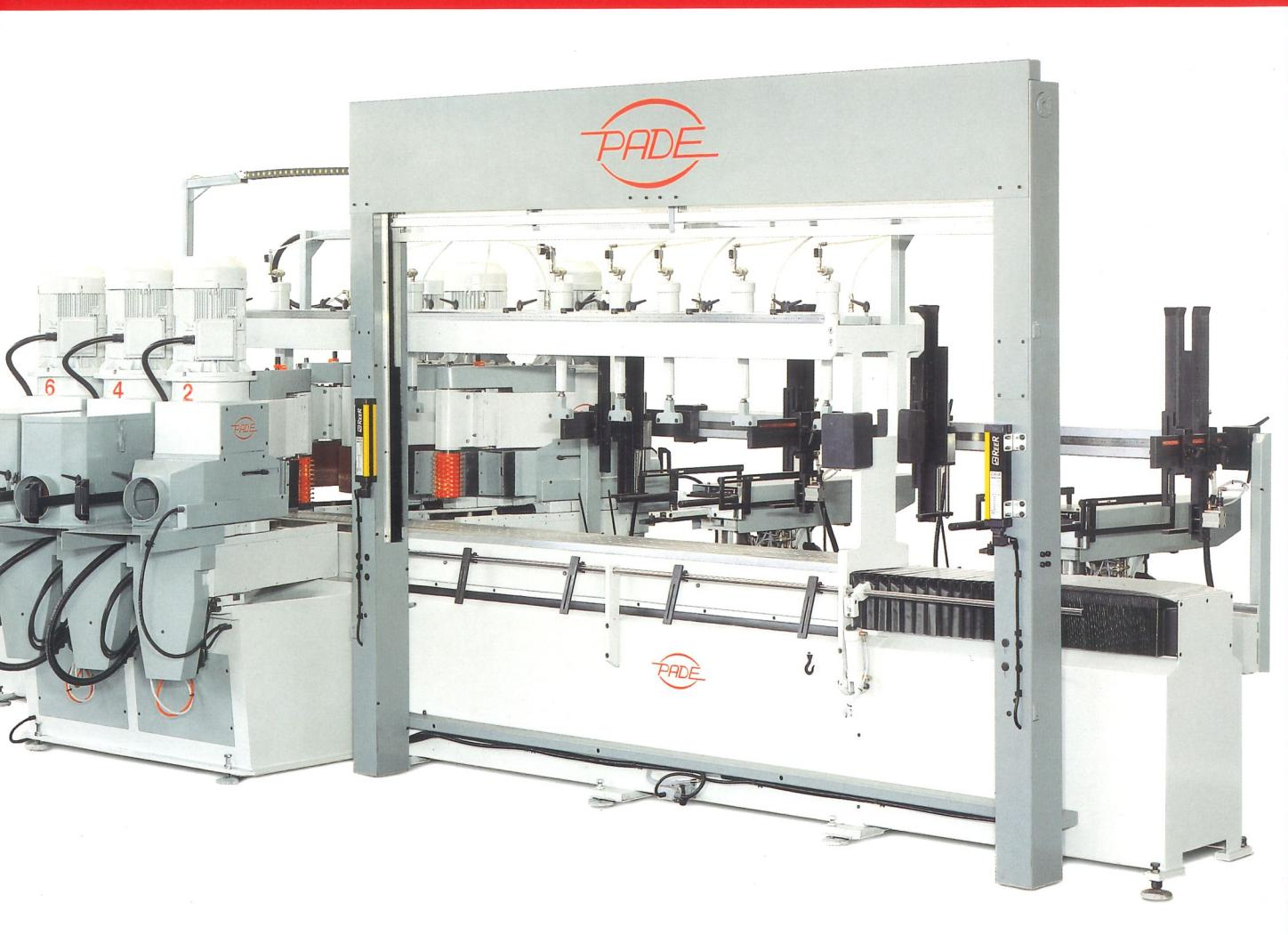
**Opening of one side of the machine (models UINZE 6T and 8T CNC)** for an easy and full access to tool change area: a hydraulic device with automatic levelling will activate rapidly and precisely the opening and closing of the unit.
