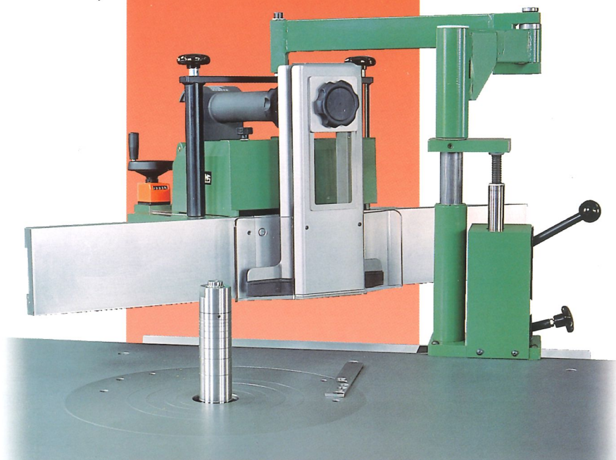
Device for pivoting the shaper fence TYP 215 and TYP 203. Option
