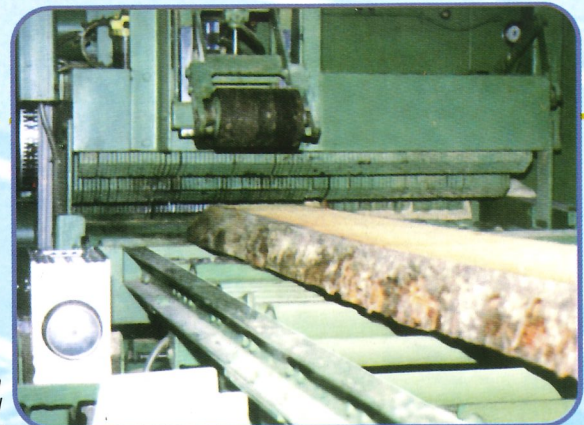
Fig. 3: Model S1200 with powered bottom infeed roller.
