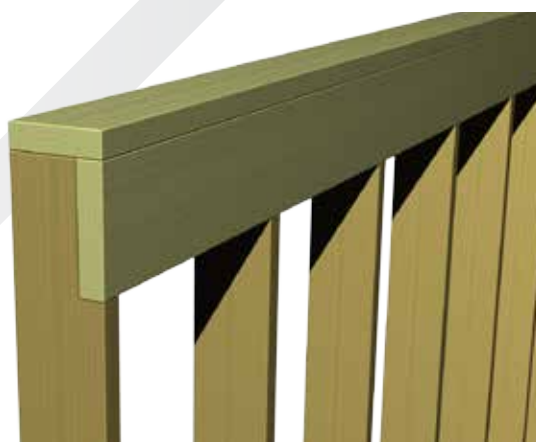
Notched studs for a wall with lintel.
