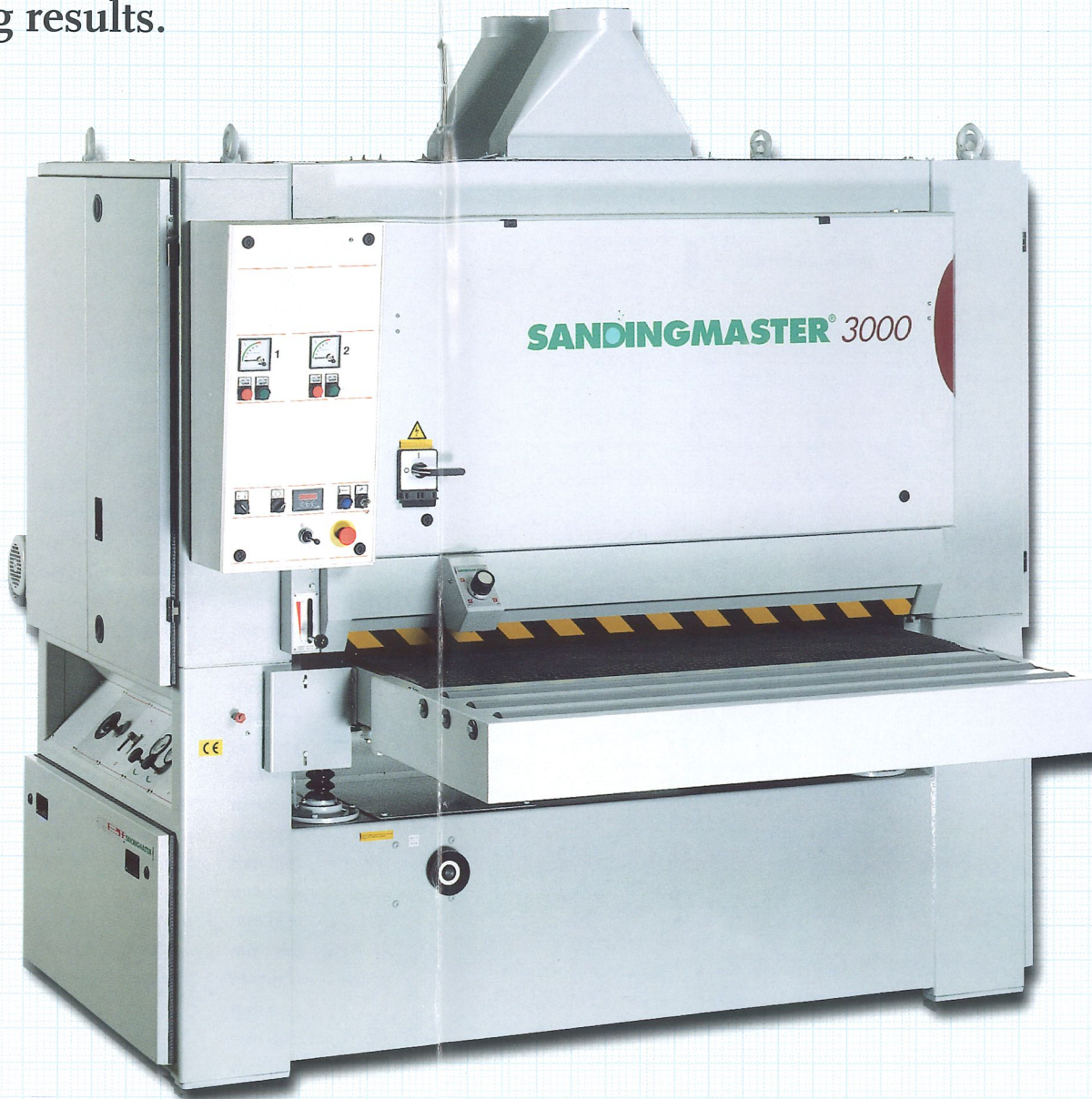
Knife planer-sander: Knife planing and wide-belt sanding in one machine. (Photo 6)
