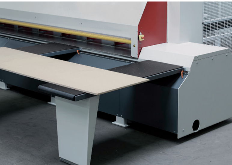
Parking position for air floatation table – for better material handling
