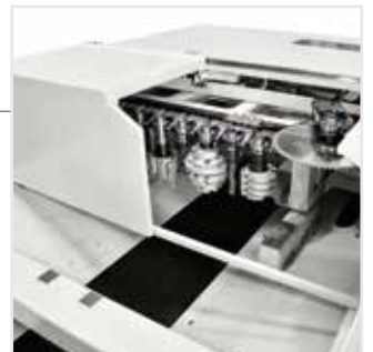
CADDY 35 tool changer, integrated in the machine footprint.
