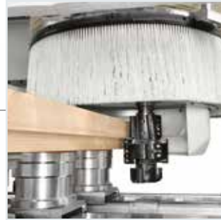
Coaxial integrated chip deflector device for maximum cleaning during machining when heavy material removal is required.
