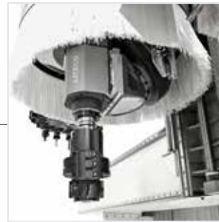
KPX 5-axis operating unit with 17kW electrospindle.
