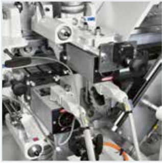
R-M trimming unit: rapid machining changeover between thin, thick and solid wood edges
