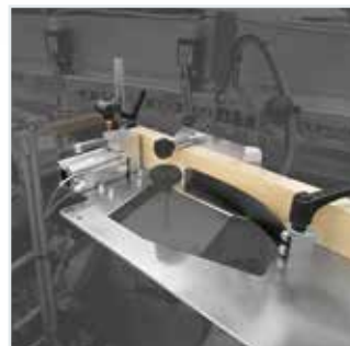
VC-M gluing unit: solid wood up to 5 mm of solid wood edge.
