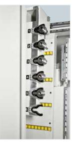
High flexibility: all the required tools always available on board thanks to the 6-positions automatic tool changer.
