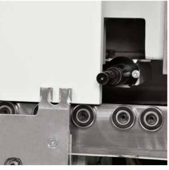
Quick and efficient panels loading thanks to the **adjustable mechanical reference stop.**
