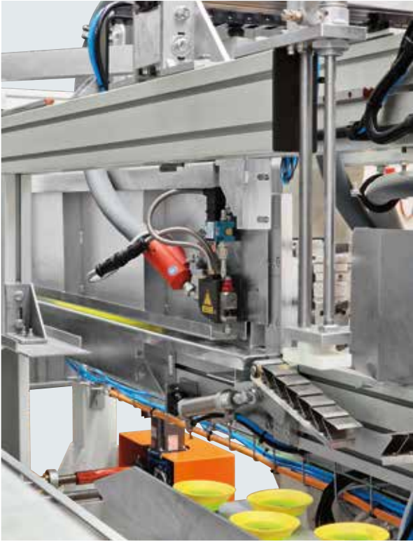
Glue nozzle and device to make the geometry of the box perfect.
