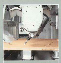
The Prisma unit revolutionises production methods and enables an innovative approach. For example, tilted tool introduction to a component and improvement in the life of the tooling.
