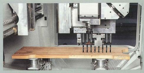
Hardware locations are directly machined by the high-powered spindle to greatly reduce cycle times.
