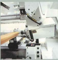
On the Prisma, holes for Anuba fittings are made using a standard drill bit. No need for angle drive heads or other special units.
