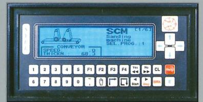
Adjustments using the electronic controller.
