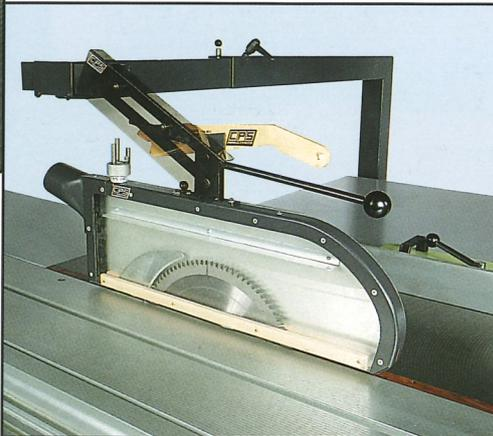
Suspended blade protection, complete with extraction outlet and height stops adjustable according to blade diameter.
