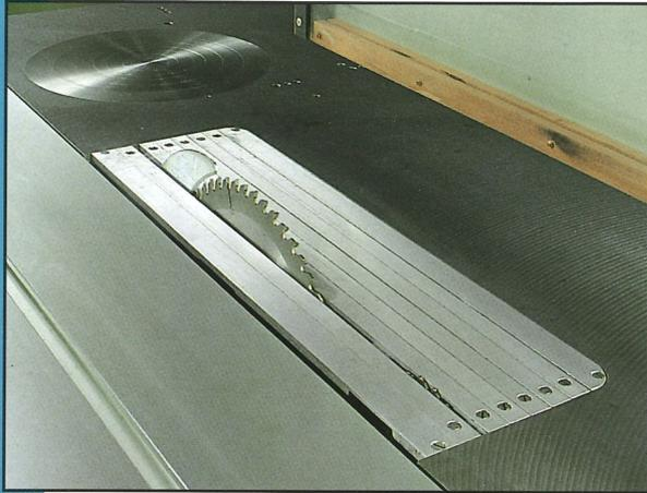
Mobile sectors on worktable enable to reduce the space necessary for the movement of the blade unit (on SI 16 T).
