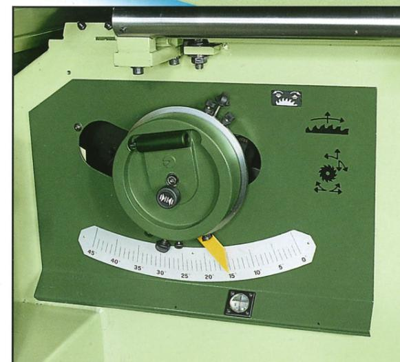
Machine set-up is quick and simple. Sideways blade adjustment is simple because of the **magnified read-out of the metric rule**.
