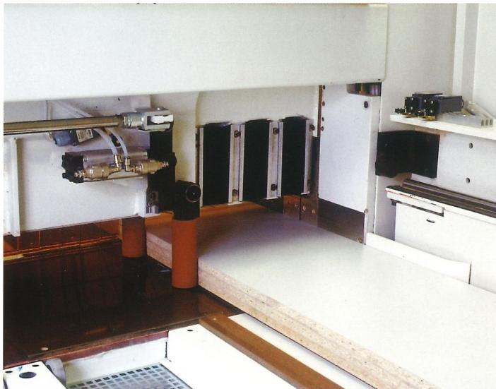
**The automatic side aligner** moves on THK-guides, reducing cutting times on cross-ways cuts and improves the finished result. A twin version with aligners (in front of and behind the cutting line) is also available on request.
