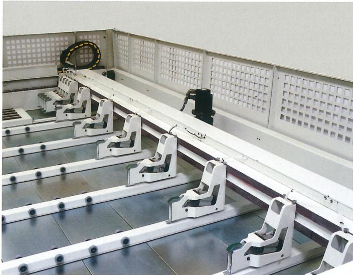
**The pusher** runs on two racks mounted on strong longitudinal H shaped beams. The reading system for the pusher positioning through magnetic band, ensures very high precision at any travel speed.
