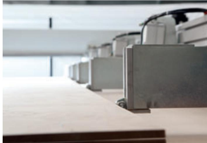
The automatic picking of the panels is executed by the grippers according to the cutting pattern requirement.
