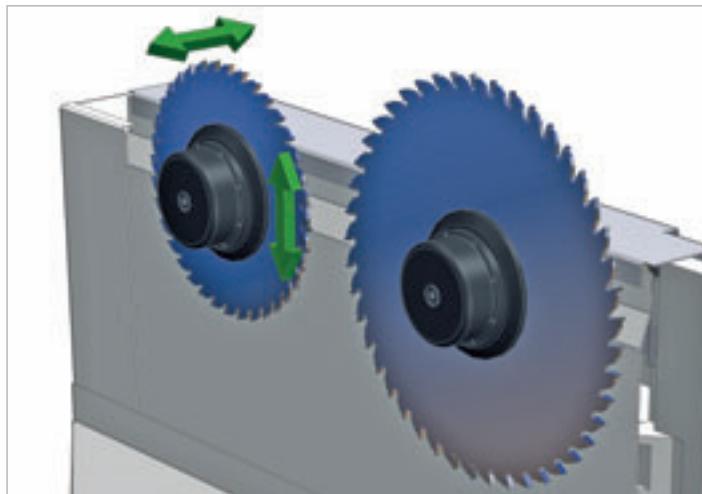
**Electronic adjustment of scoring saw blade by means of the Digiset electronic device.** This system is used to memorize and recall the aligning positions of saw blade sets, thus making extremely fast and precise the saw blades alignment after sharpening.
