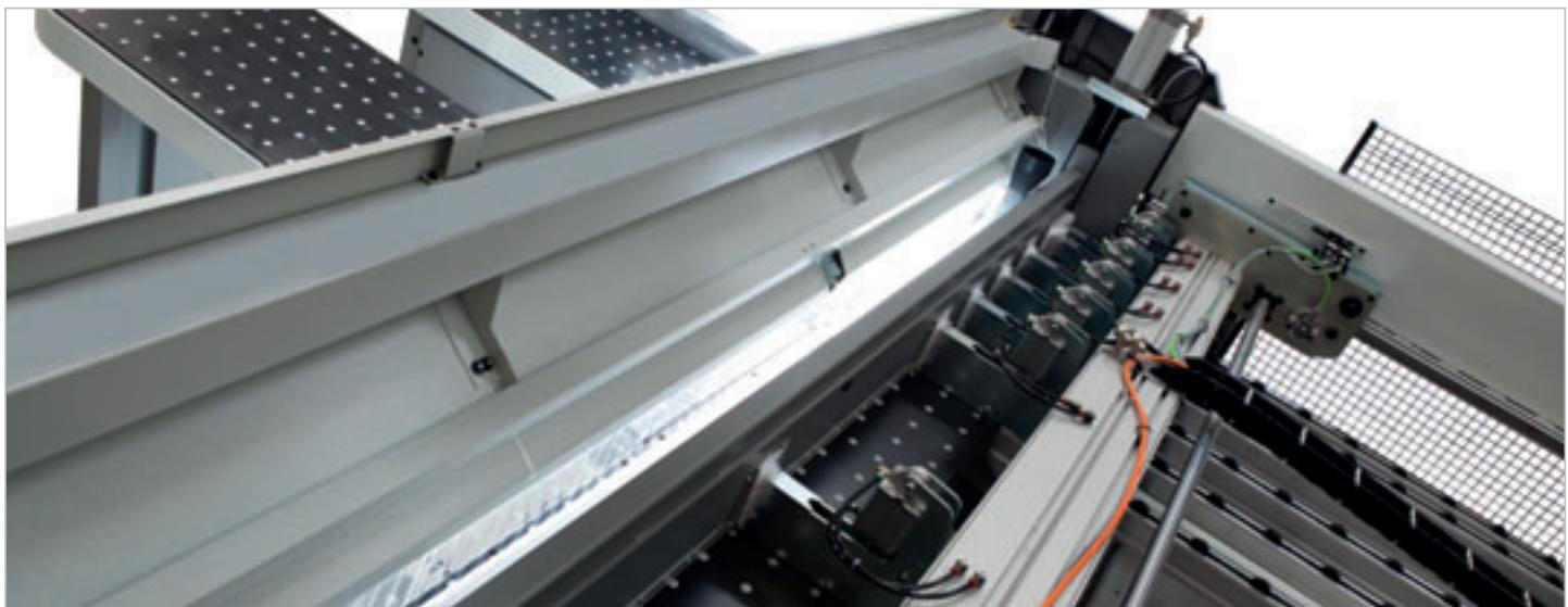
The pressure beam has a single structure for an even pressure on the stack of panels to be cut. The opening is automatically adjusted by the numerical control in relation to the thickness of the stack to be cut, thus obtaining the best cutting quality under any working condition. Not available on Sektor 450 K1.
