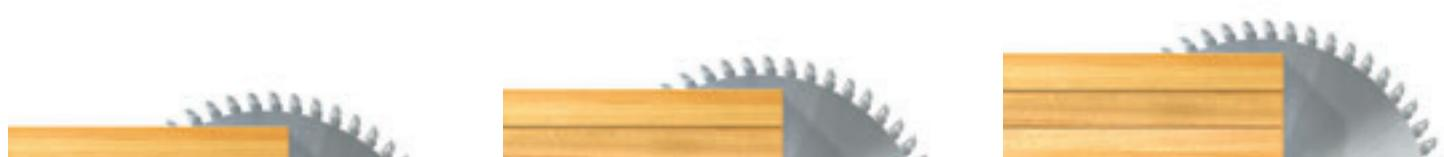
The main saw blade projection is automatically adjusted by the numerical control in relation to the thickness of the stack to be cut, thus obtaining the best cutting quality under any working condition. On the Sektor 450 K1 model the saw blade projection is automatically adjusted in two steps.
