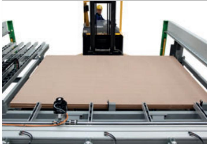
Lift table compact and integrated for automatic loading of panels, allows the loading of stacks of panels up to 500 mm directly on steel profiles. The design of the new series Sektor also provided the possibility to install the lift table as retrofit.
