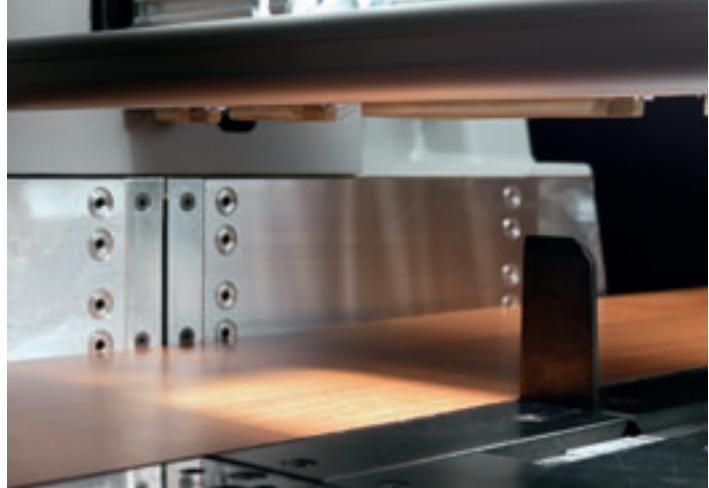
The side aligner is integrated with the saw carriage. Thanks to its characteristics, can perfectly align even thin or flexible panels, reducing cycle cutting time.
