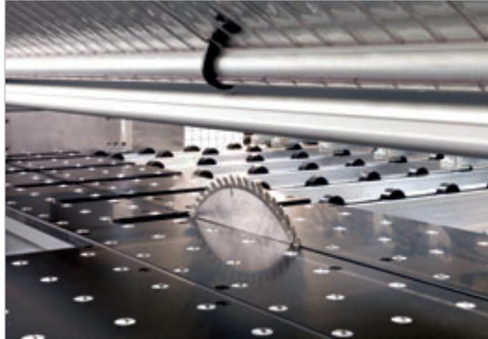
Main machine frame with air jet for gentle handling of delicate materials. It cleans as well the machine table around the blade.
