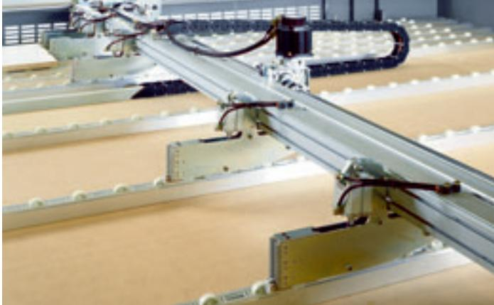
The pusher carriage for precise and fast panel positioning is driven by a brushless servomotor. The supporting table under the pusher carriage is equipped with idle independent rollers to avoid any scratching on panels with delicate surfaces.
