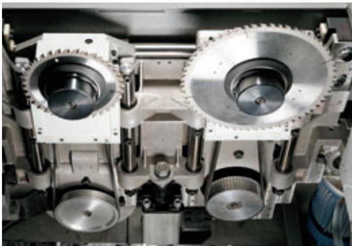
Independent raising and lowering of main saw blade and scoring saw blade is due to linear ball bushing bearings sliding on ground and hardened round bars. This system guarantees precision and rigidity to obtain a high cutting quality.
