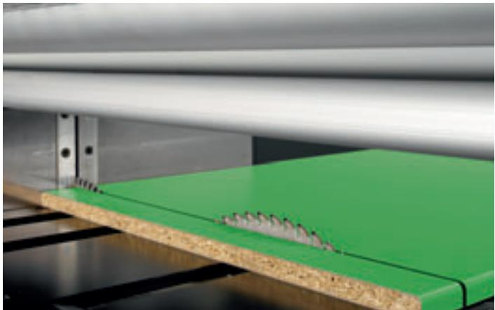
PFS device for soft and post-formed panels cut. A special numeric control program allows the perfect scoring of both entrance and exit points, avoiding the chipping of fragile and delicate material. This device is available on K2 configurations.
