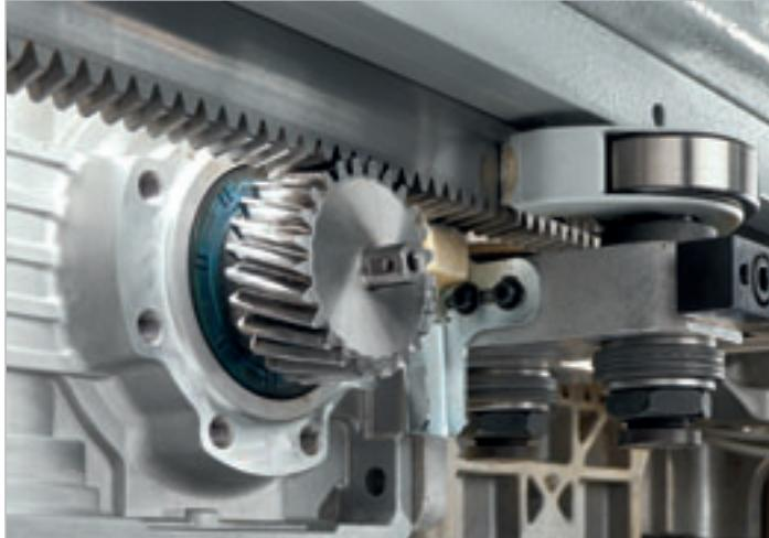
The extremely linear movement of the saw carriage is obtained by an helical rack and pinion system and by a brushless motor installed on the saw carriage itself.
