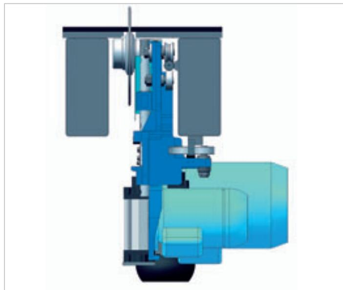
The special base structure and the positioning of the guideways and guide rollers assure an optimal weight balance of the saw carriage. The absence of saw blade vibrations is granted by the top guide which is positioned right beside the saw blade hub.
