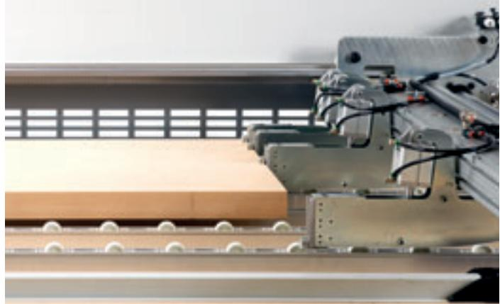
The independent self-levelling grippers assure the firm clamping of the stack of panels. Their special structure and the machine logic allow the total ejection of the stack of panel beyond the cutting line.
