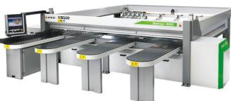
The new SEKTOR 4 series is designed and manufactured by SELCO, the brand within Biesse Wood Division specialized in panel sizing / cutting. This series of NC controlled beam saws contains technology solutions that make it suitable for small to medium sized companies as well as special departments of medium to large companies, thanks to its easy to use controls, axes
