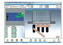
The OSI numerical control guarantees the fully automatic management of cutting patterns by optimizing all machine movements (pressure beam, saw carriage, side aligner pusher positioning, etc.). For the best cutting quality, the numerical control adjusts the optimum saw blade projection for the stack of panels being cut and sets the most appropriate cutting speed, in relation to the stack itself.
