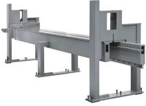
The machine base consists of a monobloc heavy duty normalized frame structure and strong supports assuring its perfect stability. The saw carriage guide ways are located on the monobloc structure, thus assuring their perfect parallelism and rectilinearity.
