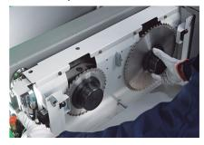
"Quick change" system for fast saw blade change (patented). Independent raising and lowering of main saw blade and scoring sawblade is due to linear ball bushing bearings sliding on ground and hardened round bars. This system guarantees precision and rigidity to obtain a high cutting quality.
