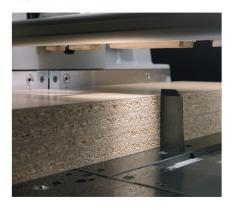
The side aligner is integrated with the saw carriage. It aligns perfectly even thin or flexible panels thereby reducing cycle cutting time.
