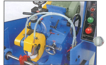
Micro-adjustment is accurate for wheel head angle.
