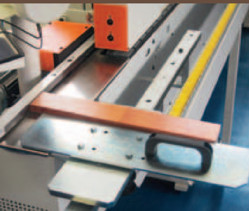
Infed system for narrow workpieces This device can be set up, facilitating the insertion of smaller panels.
