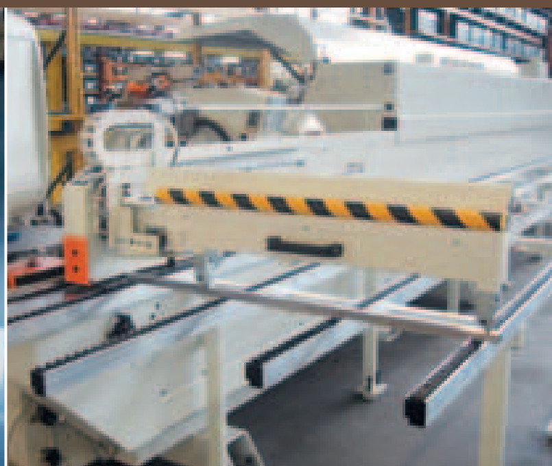
Manual infed system for large workpieces Optional device which facilitates transversal insertion of medium/large panels. The reference guide can be tilted to allow the insertion of panels with angled sides.
