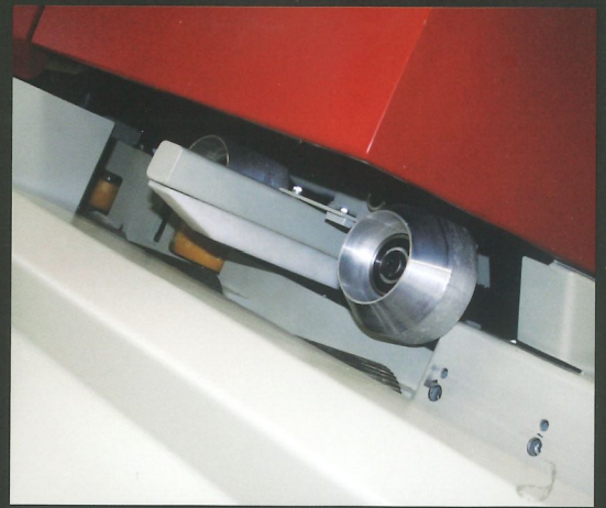
Accurate infeeding by integrated double top and bottom rollers
