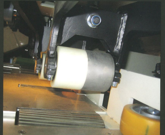
Double supported rollers for optimal workpiece contact
