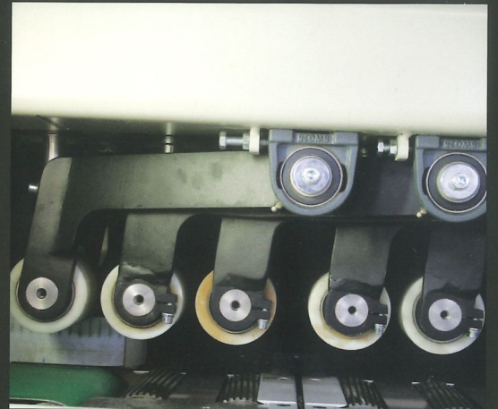
Small distance between the rollers – allowing outfeeding of short workpieces
